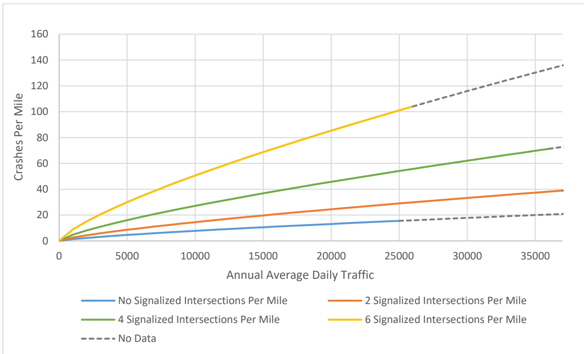
Figure 30: Crashes per Mile vs. AADT by Signalized Intersections per Mile for Total Crashes
